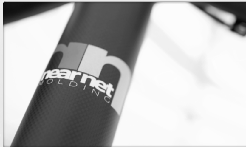
Jamis NearNet Molding technology employs a dual-molding process that yields near perfect compaction and eliminates fiber wash and wrinkles during the molding process.
