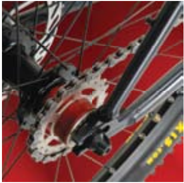
The Dragon One frame features lost wax rear entry dropouts with chain tensioning screws, slotted disc brake tabs for caliper adjustment and positioning, flush “nest”-type cable cradles with removable hose/cable retention clips, and a CNC’ed removable derailleur hanger that slides over the hub axle and fits snugly within the rear entry dropouts. With the standard cassette freehub, 21t cog and converter spacer set we’ve spec’ed, this bike can easily be converted into a lightweight geared mountain bike. Just add a rear derailleur (you’ve got one, we know), a cassette and shifter and you’re good to go. Wimp.
