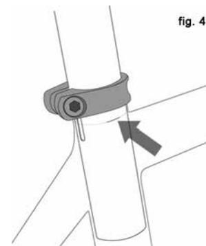
**WARNING:** If your seat post is not inserted in the seat tube as described in B.1 above, the seat post may break, which could cause you to lose control and fall.
